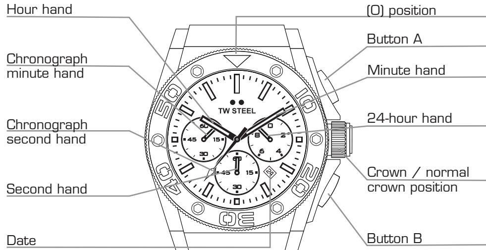
pressing button A or B. Once the hands have returned to the (0) position, return the crown to its normal position and screw the crown cap clockwise back to the case.
