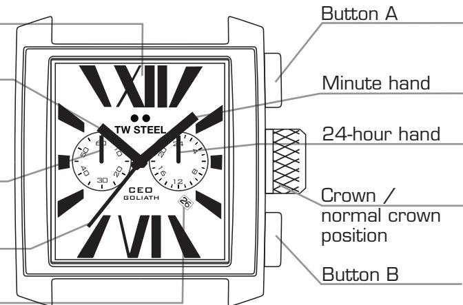
CAUTION : IF THE CROWN IS NOT PRESSED IN PROPERLY, THE WATCH IS NO LONGER WATERPROOF AND THE MOVEMENT CAN BE SERIOUSLY DAMAGED!
