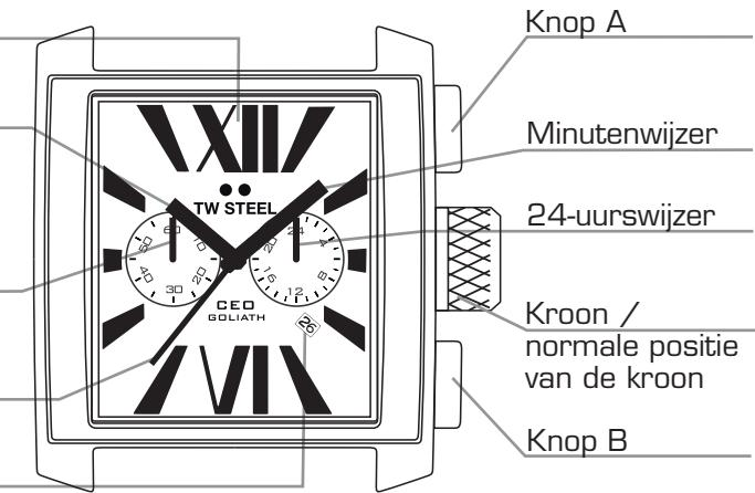
OPGELET: ALS DE KROON NIET GOED WORDT TERUGGEDUWD, IS HET HORLOGE NIET MEER WATERDICHTE EN KAN HET UURWERK ERNSTIG BESCHADIGD RAKEN!
