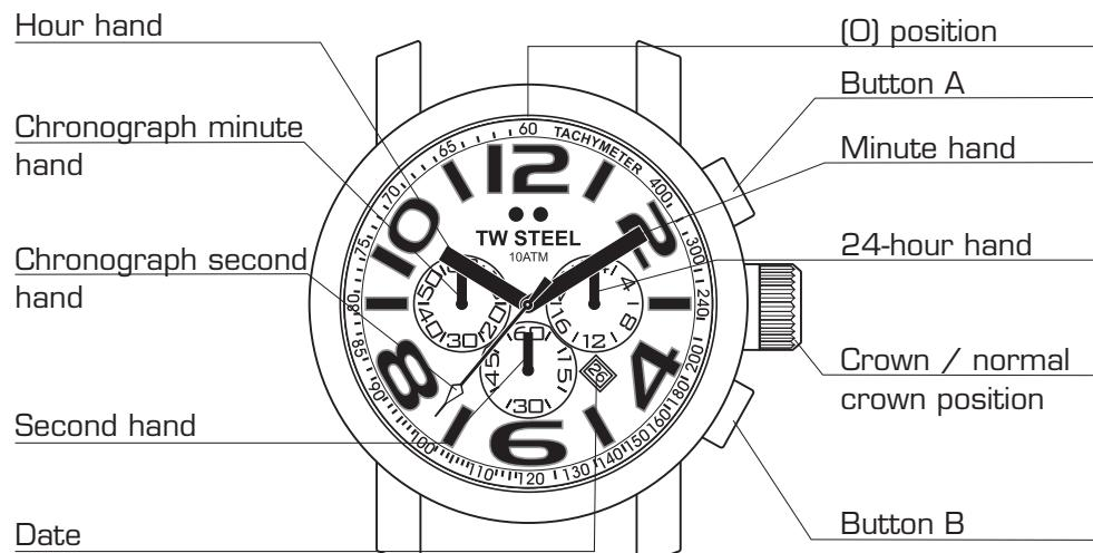
CAUTION : IF THE CROWN IS NOT PRESSED IN PROPERLY, THE WATCH IS NO LONGER WATERPROOF AND THE MOVEMENT CAN BE SERIOUSLY DAMAGED!
