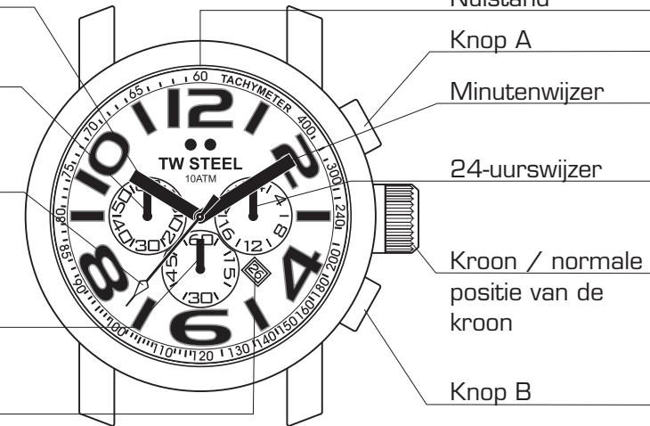
OPGELET: ALS DE KROON NIET GOED WORDT TERUGGEDUWD, IS HET HORLOGE NIET MEER WATERDICHTE EN KAN HET UURWERK ERNSTIG BESCHADIGD RAKEN!
