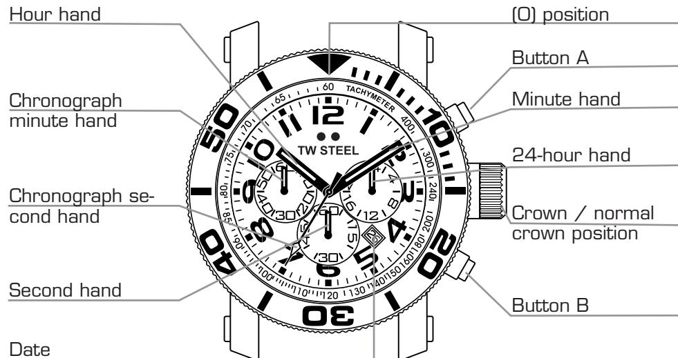
CAUTION : IF THE CROWN IS NOT PRESSED IN PROPERLY, THE WATCH IS NO LONGER WATERPROOF AND THE MOVEMENT CAN BE SERIOUSLY DAMAGED!
