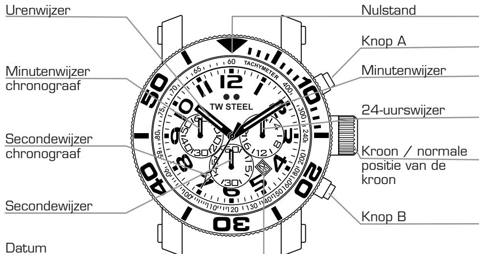
OPGELET: ALS DE KROON NIET GOED WORDT TERUGGEDUWD, IS HET HORLOGE NIET MEER WATERDICHTE EN KAN HET UURWERK ERNSTIG BESCHADIGD RAKEN!
