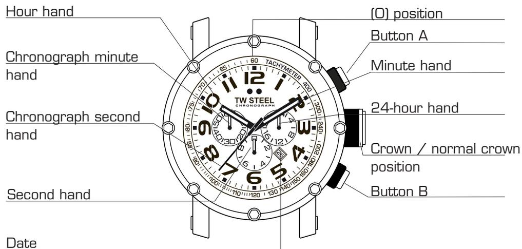
second hand to (0) position. The chronograph hands can be advanced rapidly by continuously pressing button A or B. Once the hands have returned to the (0) position, return the crown to its normal position and screw the crown clockwise back on to the case.
