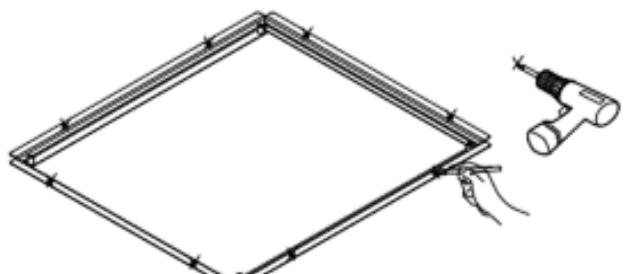
A. Do the fixed mark and drill the hole on the above which correspond to the hung ceiling frame
