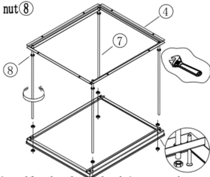
Assemble the shower head frame on the screw pump⑦, then fixed by the screw nut⑧.
