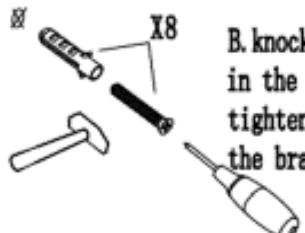
B. knock the colloidal particle in the wall, use the screw knife tightening the screw and fixed the bracket.
