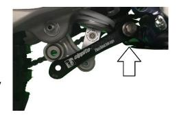
Assemble the adjustment screw of the **Fexility** on the three-point linkage.
