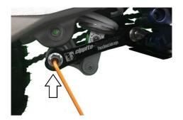
To adjust the resulting you only have to loosen the SW18 nut on the adjustment screw and unscrew approx. 4mm from its stop. After that you can then push the adjustment screw out of its locking and turn it to the desired position with the help of a 5 mm Allen key. Then push the adjustment screw back into the locking.
