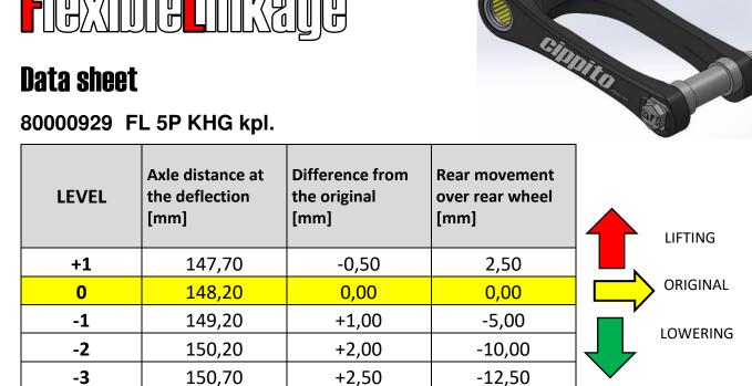
The FlexibleLinkage can be used as a replacement for the following original part:
