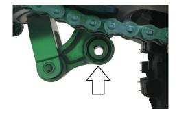
Attach the Feedball to the frame of the vehicle.
