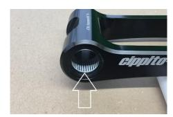
Install the original bearing bushes in the Fexille Linkage.
