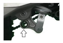
Grease the bearings and seals on the three-point linkage with a suitable bearing grease and install the bearing bush and the sealing washers of the figure in the three-point linkage.
