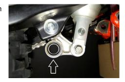
Grease the bearings and seals on the three-point linkage with a suitable bearing grease and install the bearing bush and
