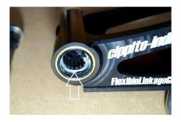
Install the original bearing bushes and sealing washers in the Fexilly Linkage.
