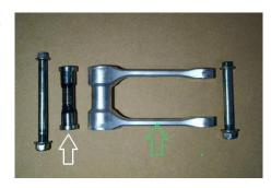
Prior to assembly, grease the bearings and seals of the flexible with a suitable bearing grease.
