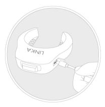
NOTE: The Lock will not charge in temperatures beyond the 0°C to 45°C (32°F to 112°F) range. The Lock will only charge when it is unlocked.
