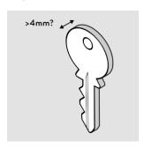
Your key doesn't fit in the Nuki Smart Lock if the "head" of the key (the part that you hold it with) is thicker than 4 mm, otherwise it won't fit in the Nuki. If a removable plastic cap is fitted to your key, remove it and then remeasure if necessary.
