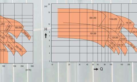
Hydraulic flow field CBH and CB at 50Hz 6 poles
