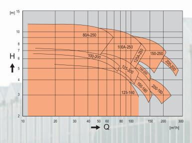
Hydraulic flow field CL and CLB at 60Hz 6 poles
