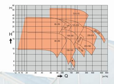
Hydraulic flow field CBH and CB at 60Hz 6 poles
