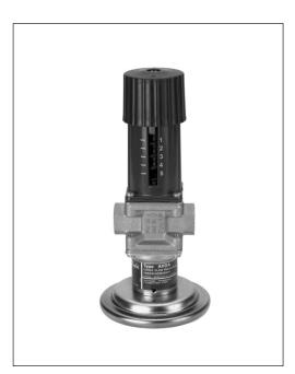
AVDA is self-acting differential pressure relief controller used for constant flow control or bypass control. Controller opens on rising differential pressure.
