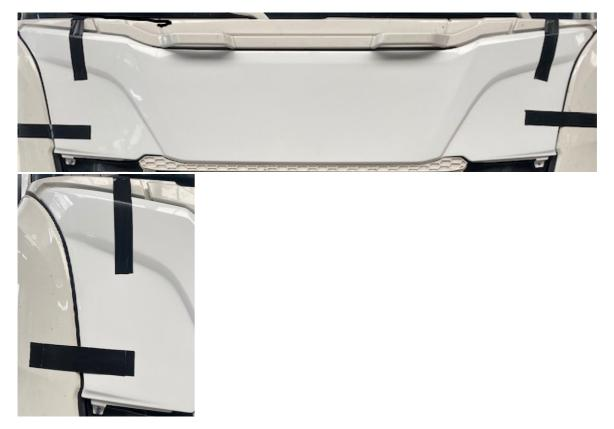
Allow this to dry for at least 4 hours before disassembling the front plate again and reinforcing and finishing the stuck supports with the supplied kit(2).
