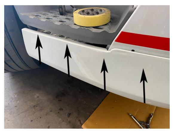
BRING THE SPOILER INTO POSITION, MOVING IT UP AND IN, THEN FIX THE 4 SCREWS INTO THE AERODYNAMIC UNDERTRAY
