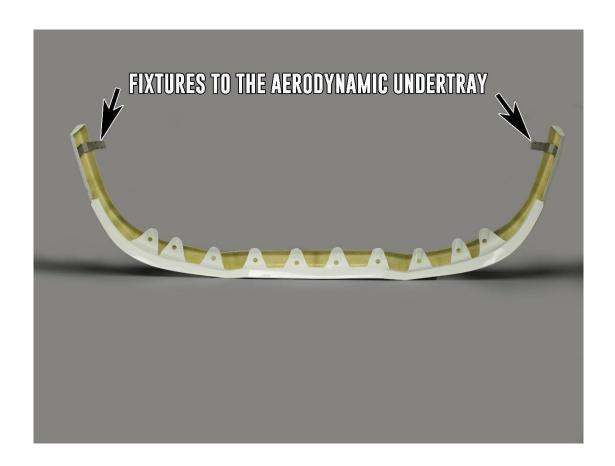
FIRST TEST FIT THE BUMPER SPOILER BEFORE PAINTING. PAINTED RETURNS WILL NOT BE ACCEPTED. THE BUMPER SPOILER IS MOUNTED ON FIXING POINTS AND CAN BE REMOVED AT ANY TIME. THE ORIGINAL UNDERTRAY BOLTS GET REPLACED BY LONGER BOLTS.
