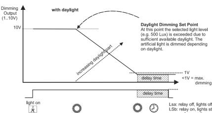
Lsa: relay off, lights off LSb: relay on, lights stays on as long as the room is occupied.
