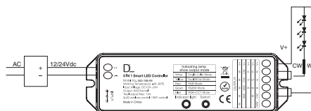
Connection of CCT LED PCBs "TUNEABLE WHITE"
