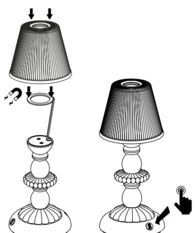
The light can be adjusted using the Lladro logo dimmer switch on the base. Just touch the logo to turn the light on.
