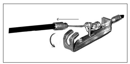
Pull the Upper Tension Connector backward and slide the wire through the slot on the bracket.
