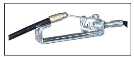
Slide the Cable wire from the Upper Tension Connector in between the opening on the wire holder on the Lower Tension Connector.
