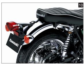
\* Front and rear fenders are formed from steel and are chrome-plated for long life and great looks, in the traditional style. Numerous other chrome parts add brilliant highpoints to complement the W800's lustrous paint. These include: the handlebar, headlamp brackets, mirrors, chain cover, shift lever, brake pedal and oil filter cover.
