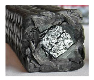
Graphite improves thermal conductivity, sliding properties and durability of the GRF.
