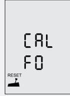
**Step5:** Push the throttle to zero position and press the “**M**” button and return to the main page.
