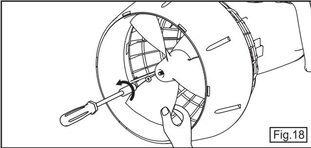
6. Slide the Propeller off the shaft, taking care not to loose the drive pin or washers.
