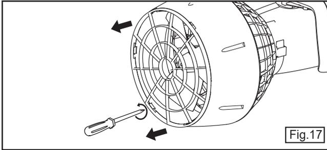
4. Unscrew the six rear grille screws as shown in figure 17.
