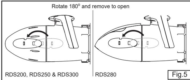
2. Remove the SEASCOOTER™ from the water, give a half turn to the Latches, remove them (see figure 5) and remove the Buoyancy Control Chamber.
