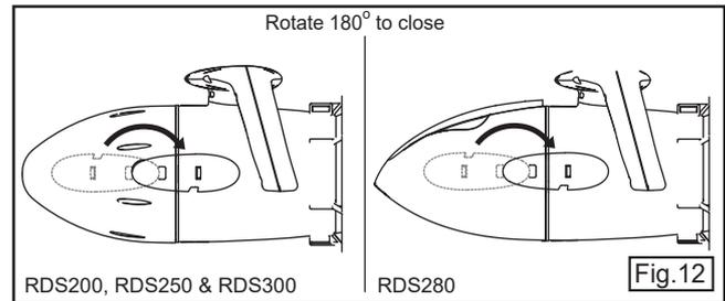
**To replace a flat battery with a fully charged battery.**
