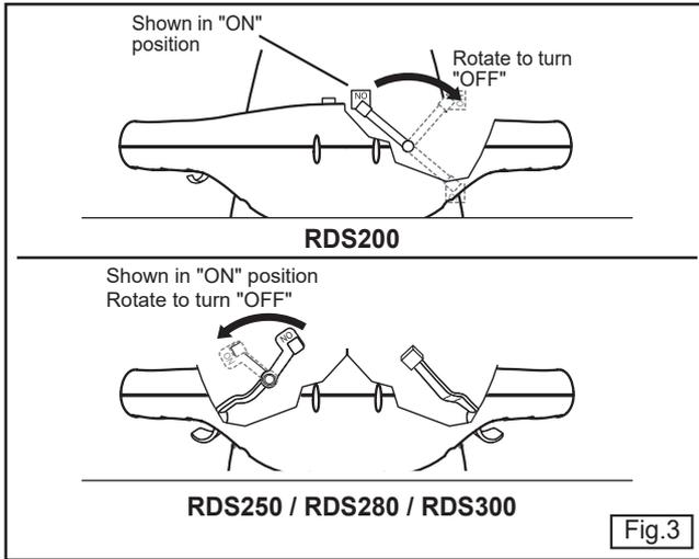
5. When ready to set off, turn the Master Switch to the On position shown in figure 3.
