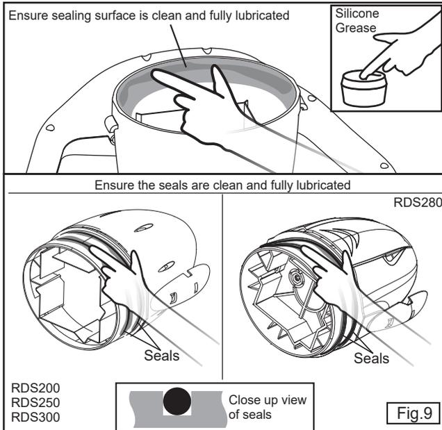
17. Make sure the seals and sealing surfaces are clean and fully lubricated with the supplied grease EVERYTIME (you can also buy this at your local hardware store) before replacing the Inner Nose Cone. See fig. 9.
