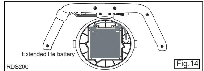
The extended battery can be charged in the same way as a standard battery.
