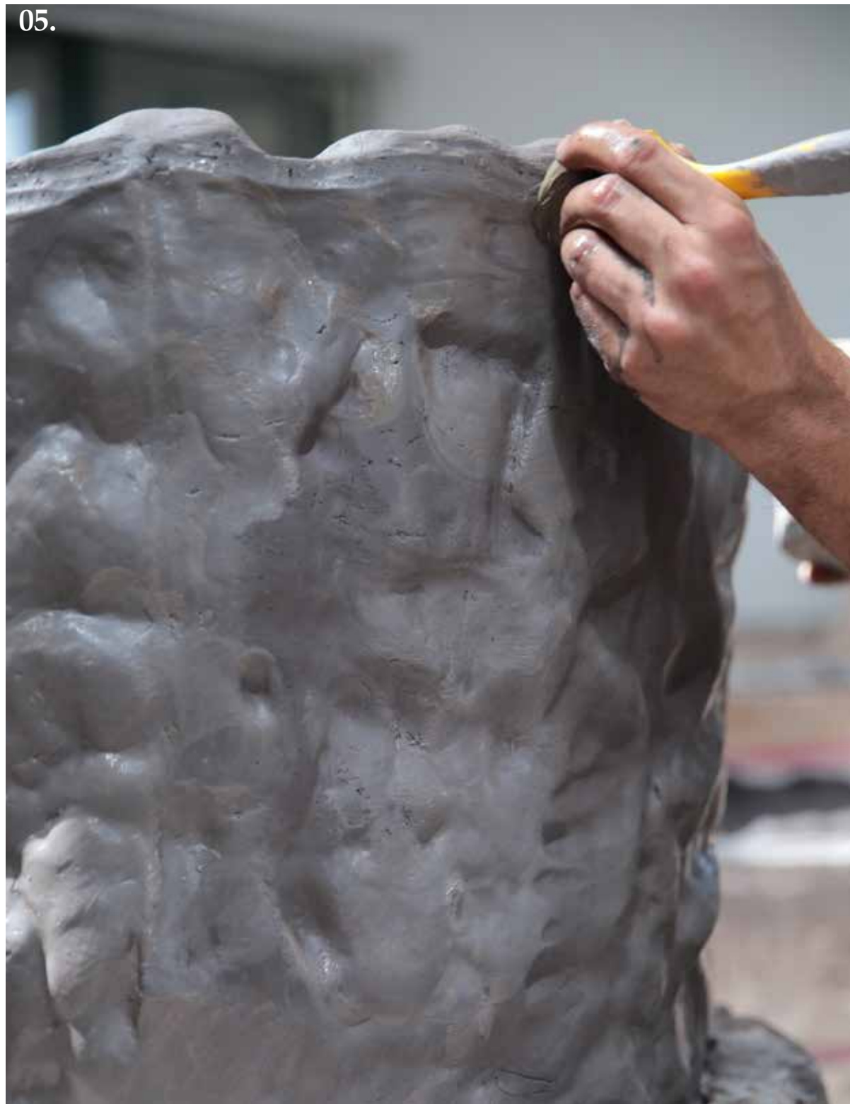
05. After removing the mould the pots need some serious cleaning and surface finishing
