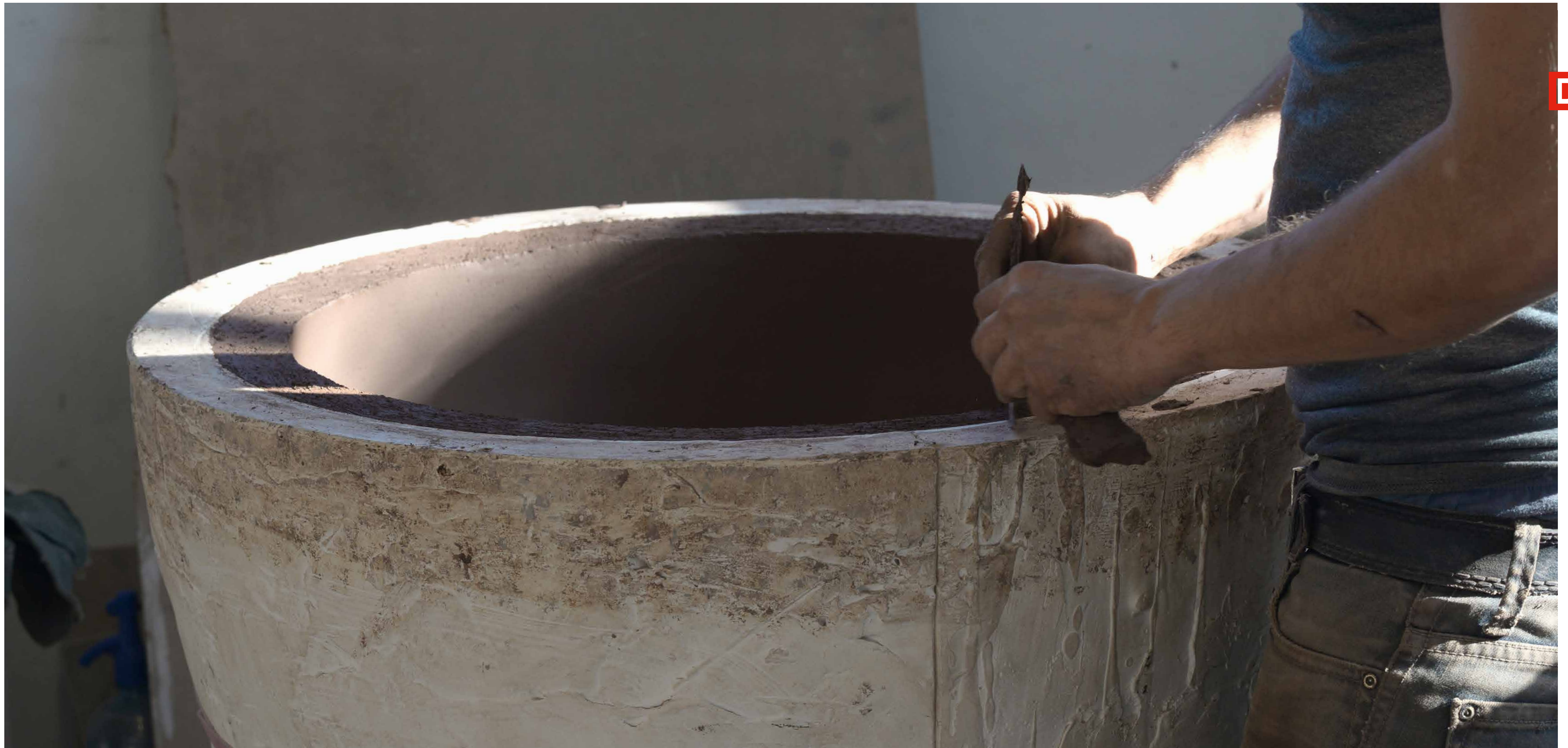
Detailing the edges after clubbing the clay into the mould
