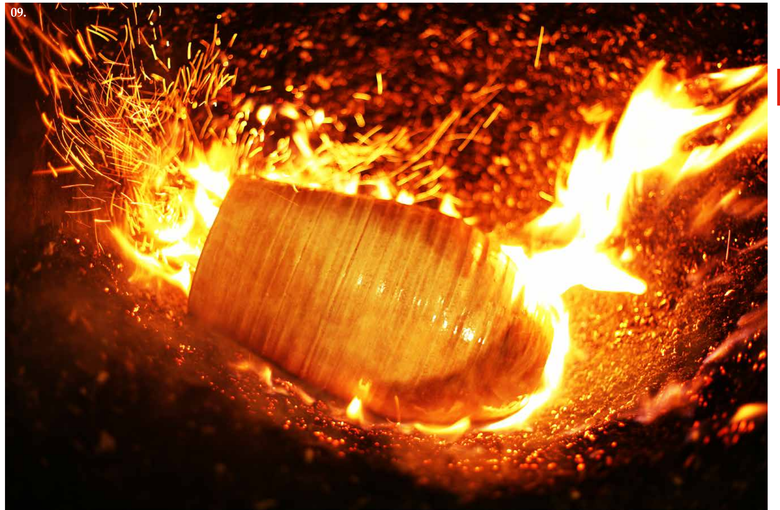
09. The pot thrust directly into a container of combustibles
