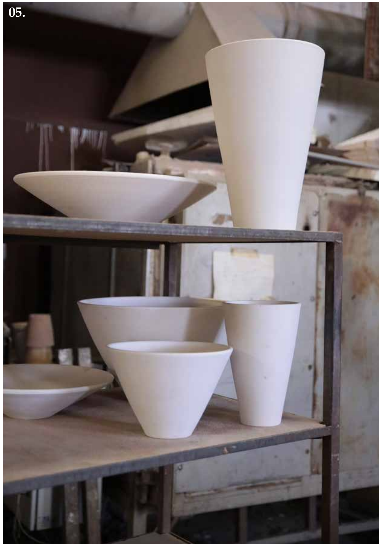
05. The bisqued pieces, after the first baking round
