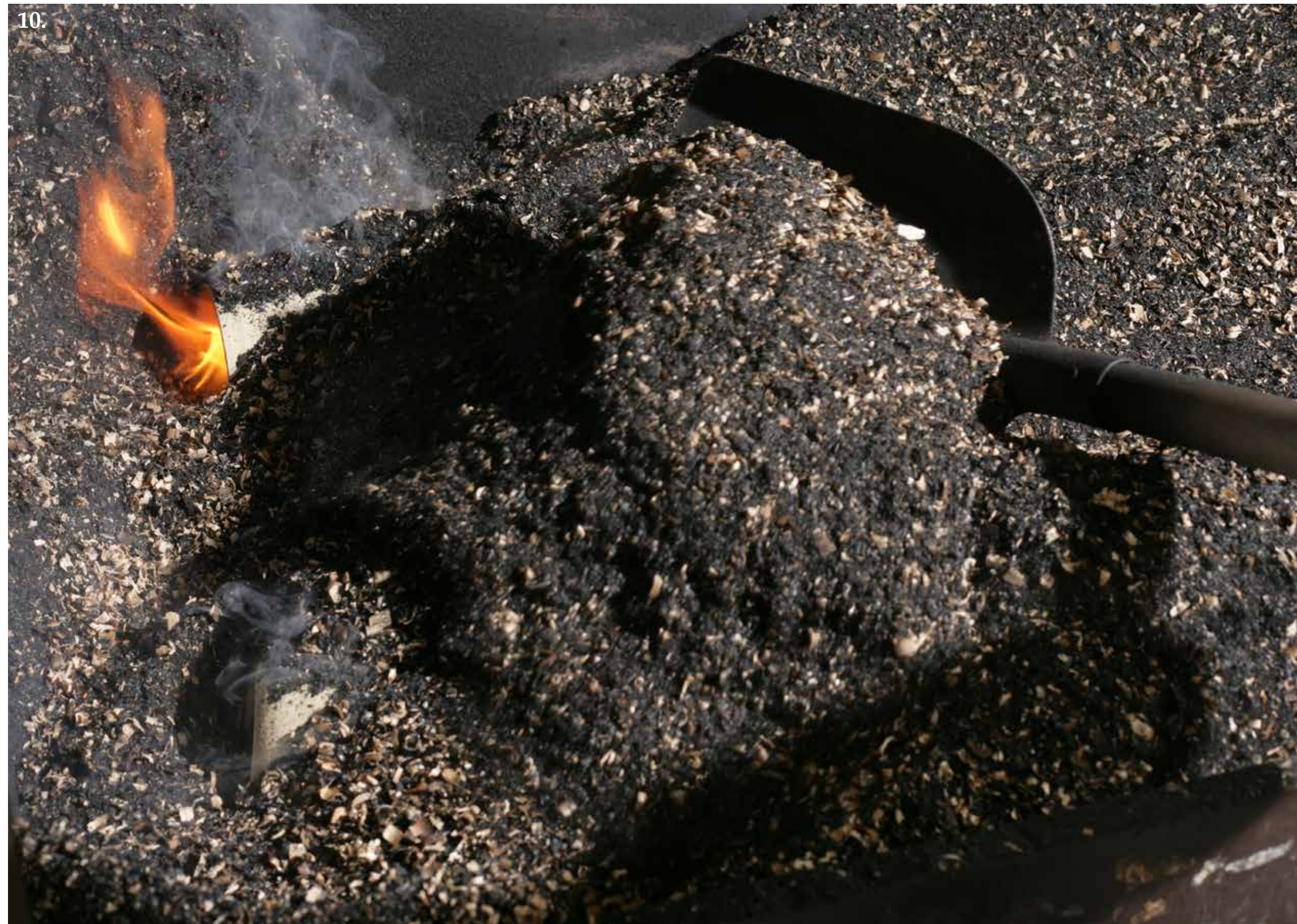
10. Throwing a lid on top of the flames to suck out any available oxygen
