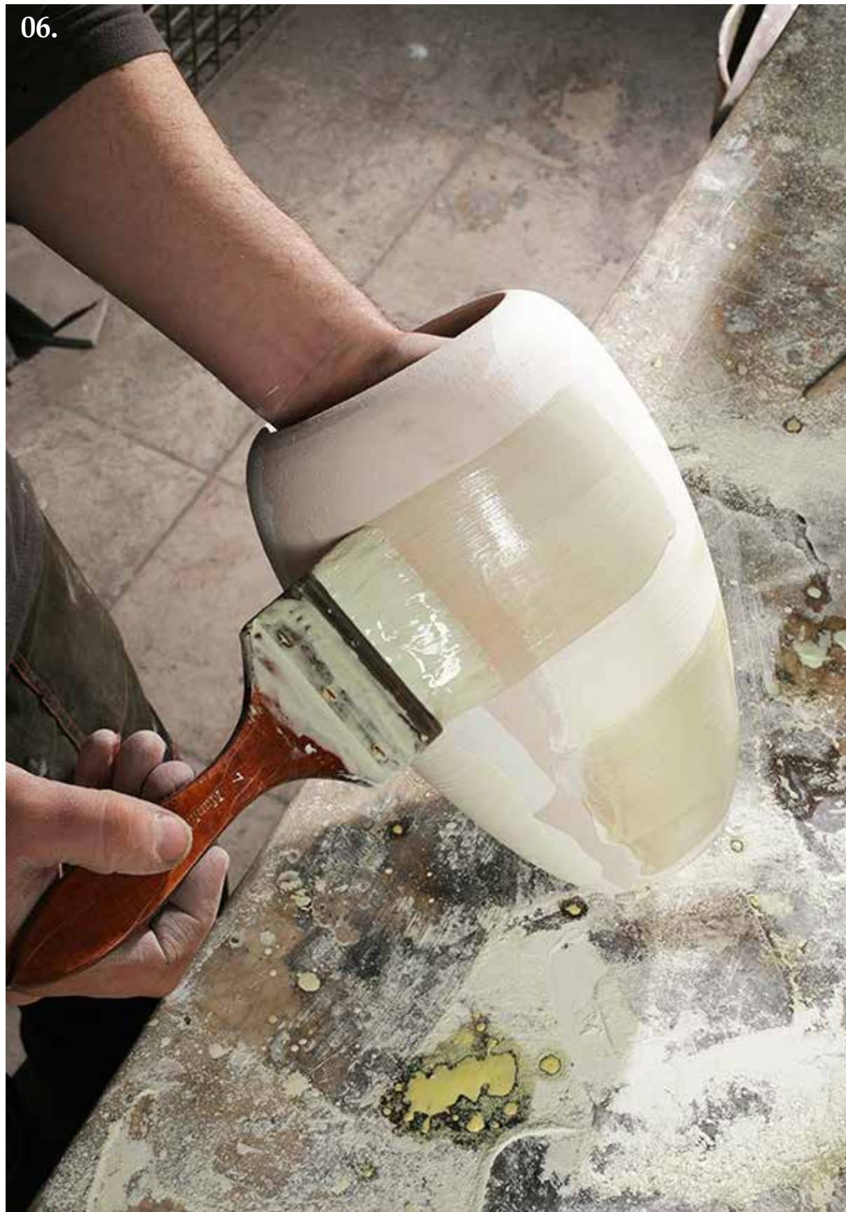
06. Decorating the bisqued pieces with stains, engobes, resist or textural treatments
