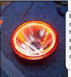
B) Place the glass carefully onto the headlight housing. Wipe away any excess silicone from the edge. Rememberto let the silicone cure long enough before installing into your vehicle application.
