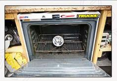
STEP # I: IN ORDER TO OPEN THE LIGHT WE WILL FIRST NEED TO HEAT THE HOUSING. IF USING A HEAT GUN BEGIN BY HEATING THE SEAL EVENLY WHILE CONSTANTLY MOVING THE HEAT GUN. IF USING AN OVEN: PREHEAT TO 225°F AND PLACE THE LIGHT IN THE OVEN FOR 10 MINUTES.
