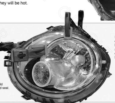
Each headlight is different if you do not like using the clamps to hold the light for curing you may also try vise-grips, ratchet straps, or any other means to hold the lens and the housing together.
