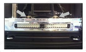
**Step 4-** Now with the Light Bars in place you can set the vertical adjustment level. Use a 13mm socket to loosen the adjustment nut and tighten once the beam is aimed at a satisfactory level.
