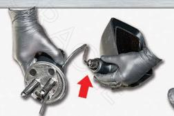
TO SEPERATE THE BASE FROM THE MIRROR, TAP SLIGHTLY ON THE BOTTOM OF THE ASSEMBLY.
