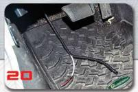
RUN A POSITIVE (+) AND NEGATIVE (-) WIRE FROM YOUR BATTERY OR 12 VOLT POWER SOURCE INTO THE CABIN.
