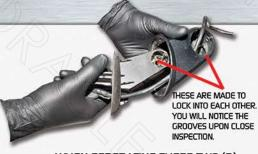
WHEN SEPERATING THESE TWO (2) PIECES, TAKE NOTE HOW THE STOCK MIRROR WIRING IS RUN. THE WIRING FOR THE LED MIRROR WILL RUN THE SAME WAY.
