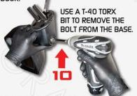
YOU CAN NOW REMOVE THE MIRROR FROM THE DOOR. TECH TIP: BEFORE PULLING MIRROR WIRES THROUGH, TIE A FISH LINE FOR RE-ROUTING THE WIRES BACK THROUGH THE DOOR EASILY.
