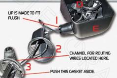
ROUTE THE LED WIRES AND THE STOCK MIRROR POWER WIRES THROUGH LOCATIONS 1,2 AND 3.
