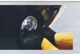
Firmly mount the fog light halo into place and press until a solid bond has formed
