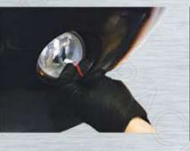
3) Fish the fog light halo wire into the wheel well
