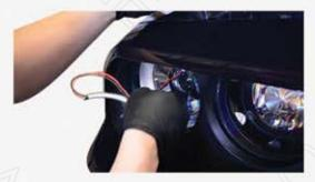
2) Start by fishing the Halo wire into the engine bay
