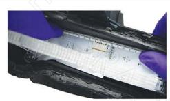
SET THE LED STRIP INTO PLACE ALONG THE HOUSING WALL. THEN PRESS DOWN **UNTIL A SOLID BOND FORMS**
