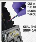
CUT A HOLE IN THE BACK OF THE HOUSING VENT & THEN ROUTE THE LED WIRING THROUGH THE HOLE
