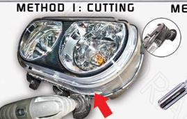
A) Use an electric multi-tool to cut into the lens. Work your way around the headlight until the lens separates from the headlight. Be careful.
