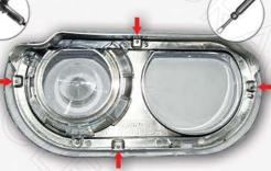
C) Remove the four (4) Phillips screws holding the chrome piece to the lens. The locations are marked with arrows.
