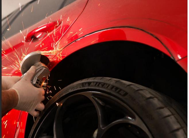
Cut the body of the car using hand cutting machine.
