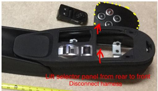
Pop out window/side mirror switch panel from underside from now removed selector panel. Disconnect harness.
