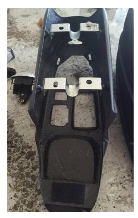
Once you have removed the center console, you have to attach 2 brackets from OEM part as seen in picture
