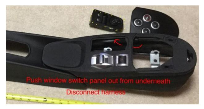
Locate the 4 10mm mounting posts with nuts. Carefully lift up that console piece and turn over to be able to access and disengage the Hazard and DNA selector harnesses. There is a guide pin at the rear of that console piece that seats and aligns that front piece with the rear piece.
