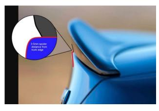
1.Before adding adhesive please check if it fits by pushing the extreme part and blocking by paper tape. If it fits good it means you can start installing it. As you seen in image distance between spoiler and edge of trunk must be **3-5mm**.
