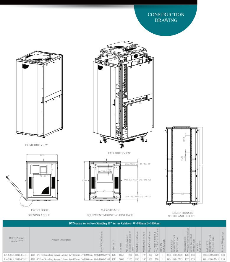
\* Please add 80mm to H mm for combined caster and leveling feet for shipping configuration.
