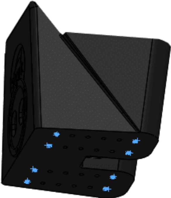
Figure 2. Plinth showing the 8 bolts used for mounting to the desk (minimum).
