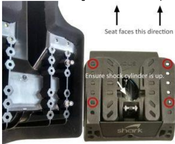
Figure 1. Seat to suspension mounting instructions.
