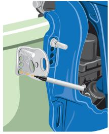
**1c.** Determine where to drill your second TurboSwing hole using the base plate as a guide.
