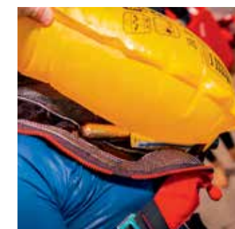
It was a shame that the rear-mounted gas bottle dug into the testers' collar bones
