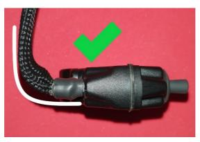
5.5. When disconnecting the Adv Ctrl cable assembly from your motorcycle or when disconnecting the magnetic sensor, never pull wires:
