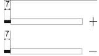
pole (-) of PV input connector. Screw two wires tightly in clockwise direction.
