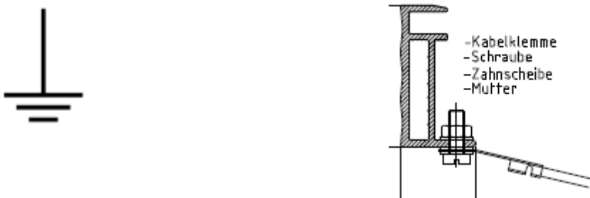
Figure 9: Equipotential bonding symbol and design
