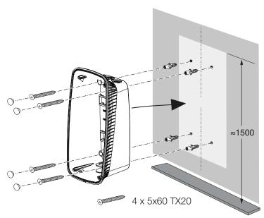
1. Screw the wallbox to the wall using screw anchors and screws. Follow the mounting instructions on the wallbox drilling template.
