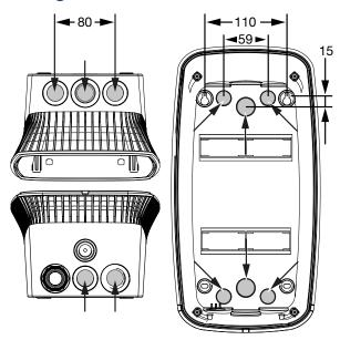
1. Use a suitable to tool to cut the required cable inlet out of the wallbox. Cable inlets are located on the rear, bottom and top.
