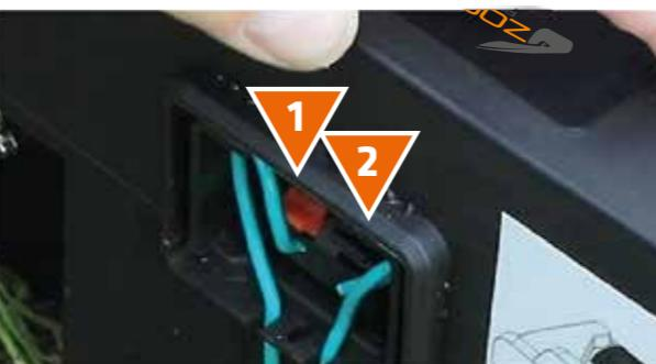
1. IN (red) - from under the docking station (end of wire).
