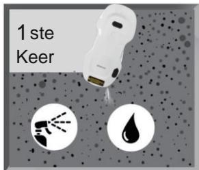
**When the robot slips, you should spray water on the cloth.**
