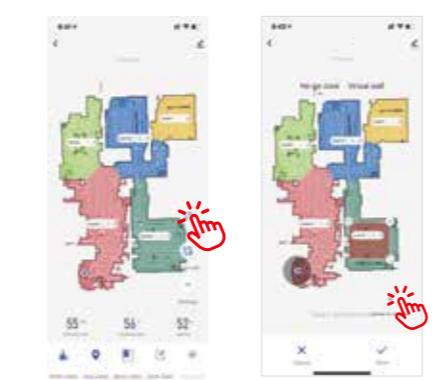
Turn on the "Y-MOPPING" button on the setting page of the APP, the robot will start mopping the floor in "Y" shape pattern.
