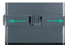
Grab and pull to open and separate the battery from unit
