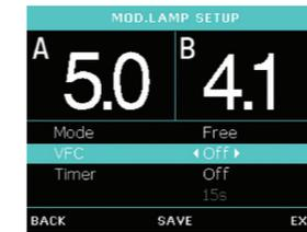
Visual Flash Confirmation. Modelling lamp shut down after flashing whilst the unit recharges.
