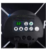
eras that give up to 7 pre-burst flashes, from simple anti-redeye to TTL preflash sequences. The power up-down can be reprogrammed to adjust in 1/10th, 2/10th, 3/10th, 4/10th, 5/10th or full EV steps. The modelling can be proprotional, full, off or proportional with minus 1 EV, to match more power-
