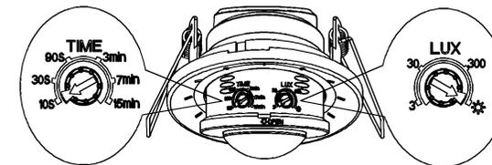
**Note: when testing in daylight, please turn LUX knob to
