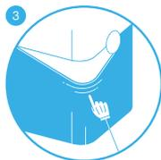
Then attach the fabric pre-filter. To ensure a smooth fit, pull it carefully over the metal frame.
