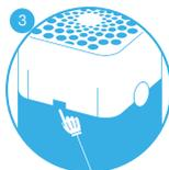
3 Before replacing the fabric pre-filter, gently press the release buttons on both sides of the unit until you hear a click.
