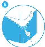
5 Re-fit the fabric pre-filter over the bottom part of the unit.
