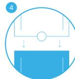
4 Firmly press the top of the unit down onto the new main filter until you hear a click.
