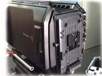
The ET-PV2UR is designed to attach directly to the rear of the URSA & URSA Mini camera bodies. Based on the popular IDX V-Plate chassis, the ET-PV2UR allows direct mounting of any IDX ENDURA Li-ion battery.
