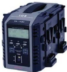
**Fully Simultaneous:** Charges up to 4 batteries at a time
